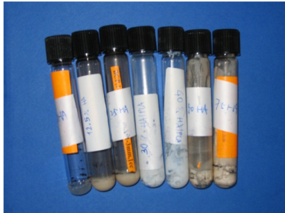
Figure 2. Loading poly(D,L-lactide) with excessively high content of apatite, i.e. more than 50%wt., led to brittle composites. In the tubes, from left to right, are the composites containing 0%, 12.5%, 25%, 30%, 40%, 50% and 75%wt. apatite content respectively. Note that the materials with 50 to 75%wt. apatite were brittle after acetone evaporation, and had many cracks..
